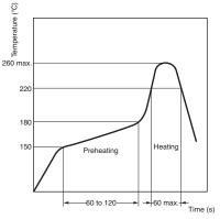
Note: The above heating curves apply if the PCB thickness is 1.6 mm.
