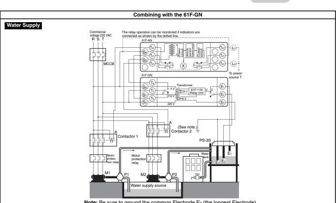
Note: Be sure to ground the common Electrode E<sub>3</sub> (the longest Electrode).
