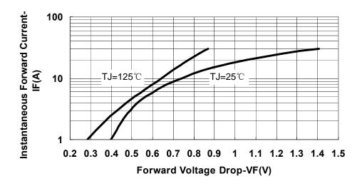
Fig.3-Typical Forward Voltage Drop Characteristics
