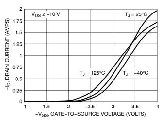
Figure 2. Transfer Characteristics
