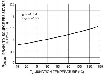
Figure 5. On–Resistance Variation with Temperature
