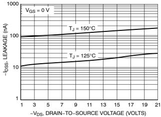
Figure 6. Drain-to-Source Leakage Current versus Voltage
