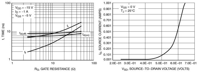
Figure 9. Resistive Switching Time Variation versus Gate Resistance
