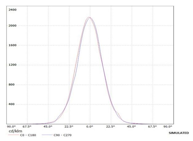
Luminaire: Ledil Oy FA11112\_LOST-M Lamps: 1 x Osram Ostar lighting plus 250mA 283lm 3000K
