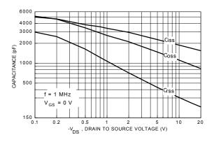
Figure 9. Capacitance Characteristics.
