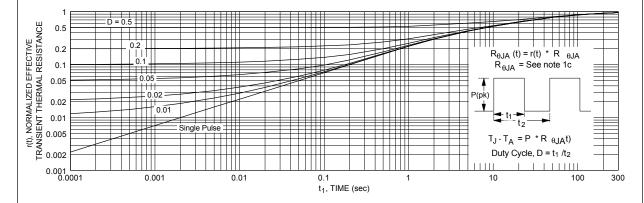
Figure 17. Transient Thermal Response Curve.
