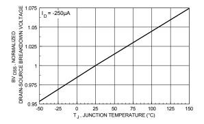
Figure 7. Breakdown Voltage Variation with Temperature.
