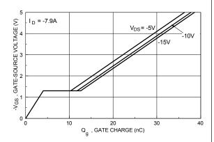
Figure 10. Gate Charge Characteristics.
