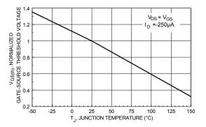
Figure 6. Gate Threshold Variation with Temperature.
