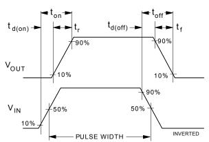
Figure 12. Switching Waveforms.
