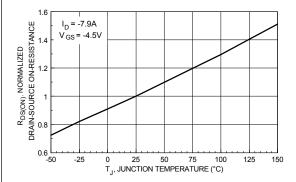
Figure 3. On-Resistance Variation with Temperature.
