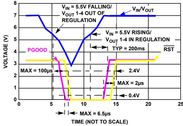
FIGURE 1.  $\overline{PGOOD}$  AND  $\overline{RST}$  TIMING
