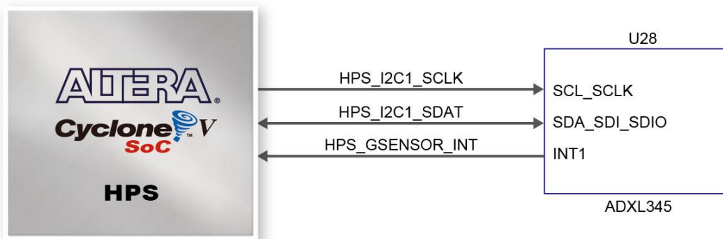
Figure 3-38 Connections between Cyclone V SoC FPGA and G-Sensor
