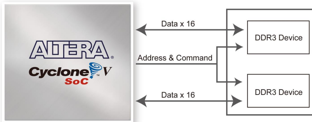
Figure 3-35 Connections between FPGA and DDR3
