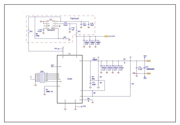
Fig. 3 - Reference Design Schematic
