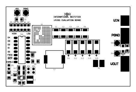
Fig. 4 - Component Placement (Top View)
