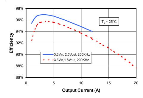
Fig. 2 - Typical Efficiency vs. Current
