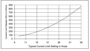
Fig. 6 Current Limit Adjustment using  $R_{LIM}$
