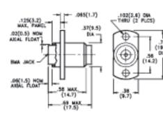
SPECIFICATIONS Impedance: 50 Ohms Frequency: DC - 18.0 GHz VSWR: 1.10 + 0.01 (f GHz) Power: 0.5 Watts max @ 25 °C Operating Temperature Range: -65 to +125 °C Finish: Passivated Stainless Steel
