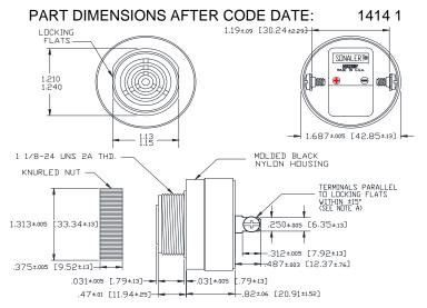
NOTE A: TERMINALS-.032 BRASS TIN PLATED, TAPPED FOR #6-32 SCREW. TWO #6-32 NICKEL PLATED BRASS SCREWS INCLUDED. WILL ACCEPT 1/4" QUICK CONNECT. NOTE B: MOUNTING- REMOVE BLACK PLASTIC NUT
