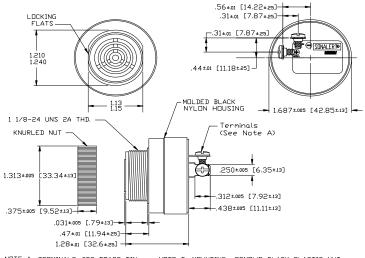
NOTE A: TERMINALS-.032 BRASS TIN PLATED, TAPPED FOR #6-32 SCREW. TWD #6-32 NICKEL PLATED BRASS SCREWS INCLUBED. WILL ACCEPT 1/4\* QUICK CONNECT. TE B: MOUNTING- REMOVE BLACK PLASTIC NUT AND INSERT THREADED FRONT THROUGH 1.25' HOLE PUNCHED IN PANEL, IF DRIENTATION IS NEEDED, NOTE LOCKING FLATS ON DRAWING. SCREW NUT BACK ON. DO NOT OVERTIGHTEN.
